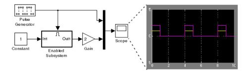
Simulink software computes the outputs of the Constant block and Gain Block only when the Enabled Subsystem executes (i.e., at time steps 0, 4, 8, and so on). This is because the output of the Constant block is required and the input of the Gain block changes only when the Enabled Subsystem executes. When CE behavior is off, Simulink software computes the outputs of the Constant and Gain blocks at every time step, regardless of whether the outputs are needed or change.
