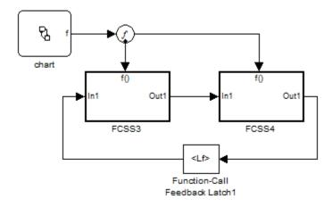
In either case, the latching results in the destination block reading a delayed signal from the previous execution of the source function-call block.
